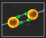
1. Splitting O2 The ZERO3® AO Generators split Oxygen (O2) molecules into single radical Oxygen (O1) atoms via the corona discharge. creating Ozone (O3).
