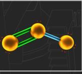
2. O<sub>2</sub> Becomes O<sub>3</sub> The single radical Oxygen (O1) atoms bond to remaining Oxygen (O<sub>2</sub>) molecules,
